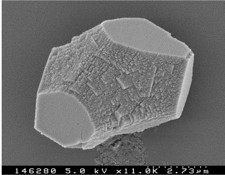
Figure 3 Calcium carbonate crystals from the raw water.
